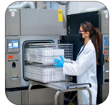
LSO Technician loading a 3M™ Steri-Vac™ Sterilizer to initiate an ethylene oxide sterilization cycle.
