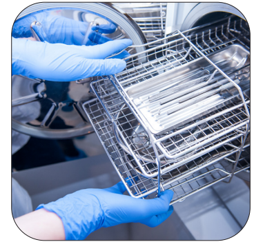
Technician collecting surgical tools following a steam sterilization cycle.
